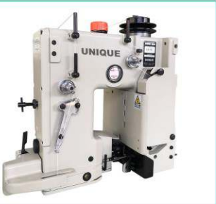
DS-9C/GK95-1 High speed 1 needle 2 thread bag closing machine Speed: 2700 rpm Stitch length: 7-10.5mm
