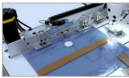
Automatically switch out the corresponding sewing program through RFID electronic radio
