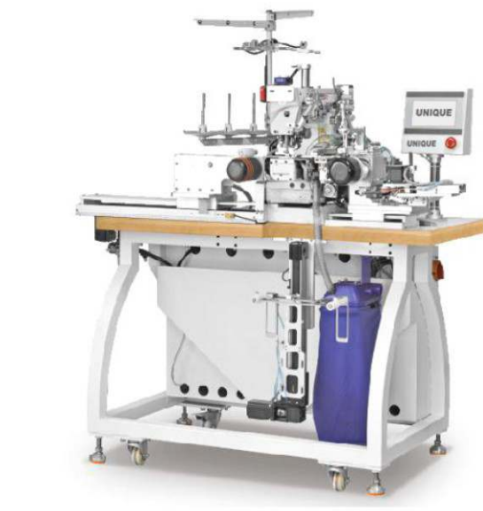
GK-346-3 Automatic coverstitch machine for tunnel elastic waistband
