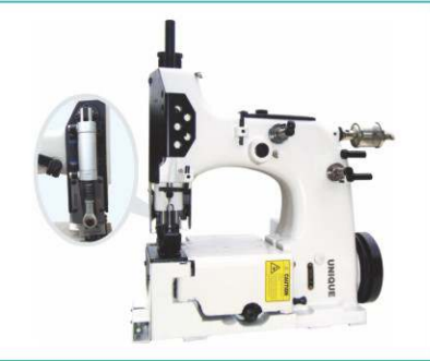
GK35-7 1 needle 2 thread bag closing machine (Pneumatic thread cutter) Speed: 2000 rpm Stitch length: 6.5-11mm Max thickness: 8mm
