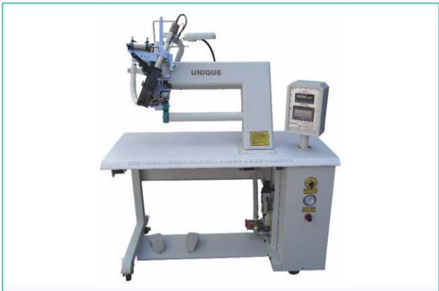
UN-HS-A6 Hot air seam sealing machine Max temperature:700℃ Roller width:25.4mm Applicable tape width:14-22mm
