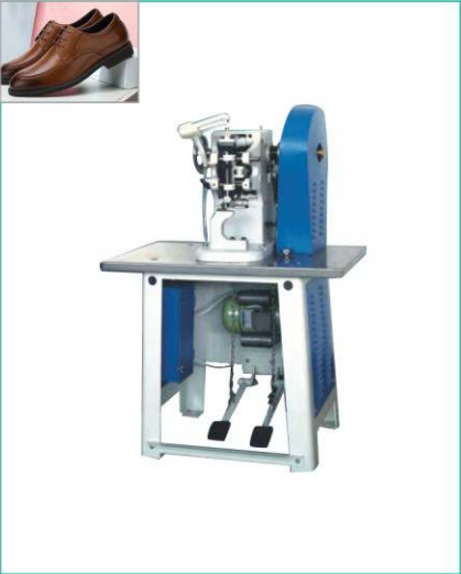
UN-PH30 Automatic leather punching hole machine
