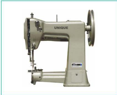
GR1-8-1 Max thickness: 40mm Working area: 190*240mm Stitch length: 8-12mm Speed: 400 rpm Presser foot height: 15/40mm
