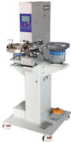
UN9815 AB Snap button - cover CD Snap button - bottom CD-S Snap button with auto gasket filling
