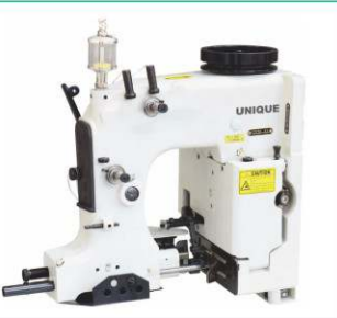
GK35-6A High speed 1 needle 2 thread bag closing machine GK35-6A: basic type GK35-6AF: left side of GK35-6A Speed: 2000 rpm Stitch length: 6.5-11mm Max thickness: 8mm
