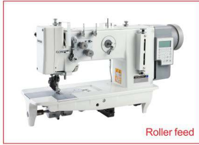
GC287D-273 Computerized roller feed 2-needle lockstitch sewing machine
