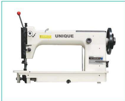
UN255 Stitch length: 14mm Speed: 1200 rpm Extra large hook Up and down feed
