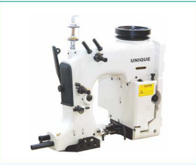
GK35-2C/80800 1 needle 2 thread bag closing machine Speed: 1900 rpm Stitch length: 6.5-11mm Max thickness: 8mm
