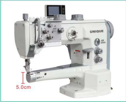
UN669-180312-7/P Computerized compound feed cylinder bed lockstitch sewing machine with auto trimmer, back-reverse stitch and pneumatic foot lifer UN669-180312-P direct drive with auto back-reverse stitch and pneumatic foot lifer
