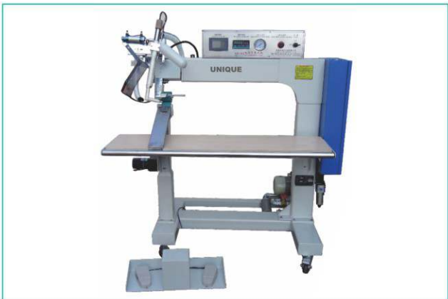
UN-HS-A8 Hot air seam sealing machine Max temperature:700℃ Roller width:30mm Applicable tape width:14-25mm
