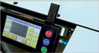
Buttons + full LCD touch screen, USB program input
