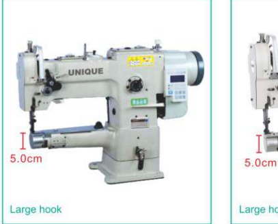
UN246D-P Direct drive cylinder bed compound feed lockstitch sewing machine with auto foot lifter and back reverse stitch
