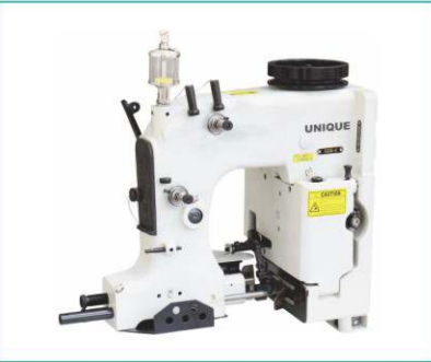
GK35-6 1 needle 2 thread bag closing machine with auto thread cutter Speed: 1900 rpm Stitch length: 6.5-11mm Max thickness: 8mm
