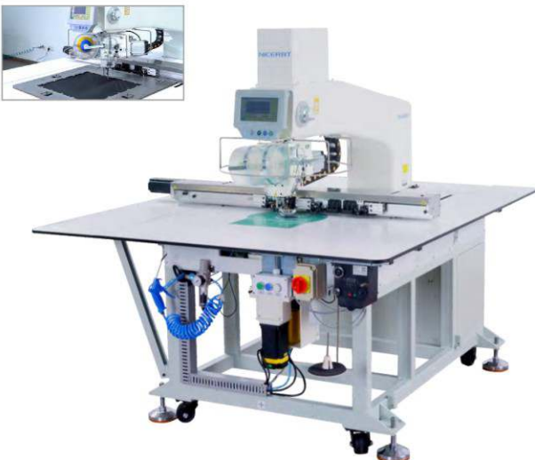
UN8400A-6055H-D (600x550mm) Rotary head for leather sewing
