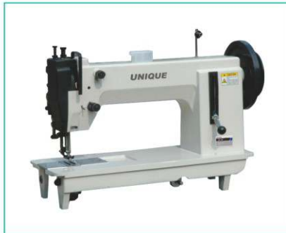
GB6-181 Working area: 200*420mm Stitch length: 12mm Speed: 800 rpm Presser foot height: 13/22mm Up and down feed
