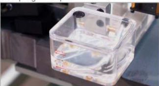
Rotary hook adopts oil-line lubrication
