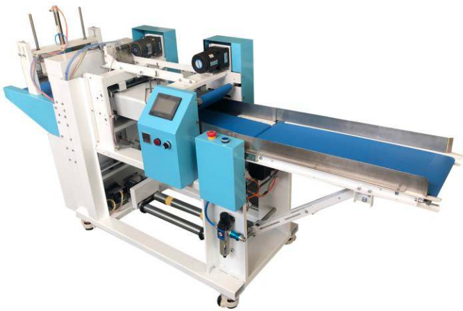
UN-P308C 3 sided seal bagging machine UN-P308C for light like shirt,towel UN-P309B for heavy like winter clothes, pillow
