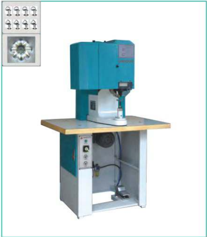
UN-CS908 Climbing shoes button attaching machine
