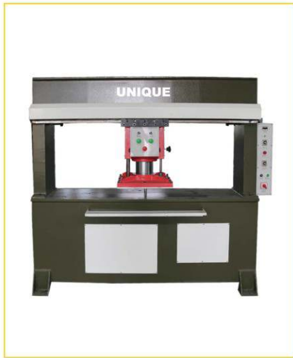
UN-250KN Hydraulic movable head die cutting machine
