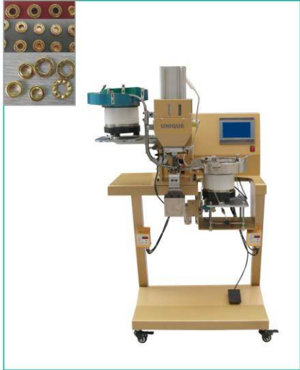
UN-EH-98A Automatic double side eyelet punching machine
