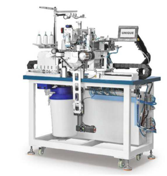
GK-375S Automatic underwear elastic waistband attaching machine
