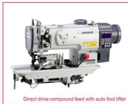
Direct drive compound feed with auto foot lifter
