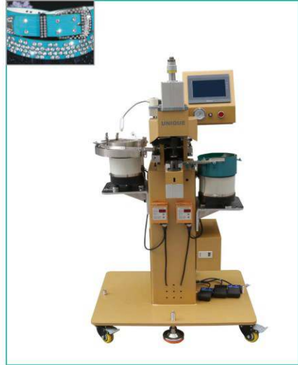
UN-198-8B Automatic hollow nail (with rhinestone) up-down rivet attaching machine
