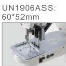
UN1906ASS Electronic bar tacking machine with 60*52mm
