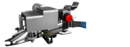
OPTIONAL Hot cutter for binding tape with feeding roller
