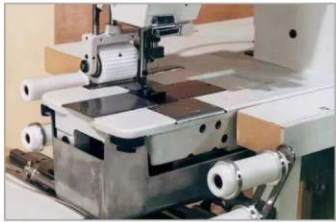
Option 1: rear puller - plastic & gear type Option 2: rear puller - rubber & flat type Option 3: extension rollers for waist-band sewing
