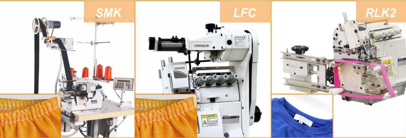
SMK: Elastic attaching Electric metering type elastic tape feeding EX5114DD-SMK EXT5114DD-SMK GN901D-4-SUT-SMK
