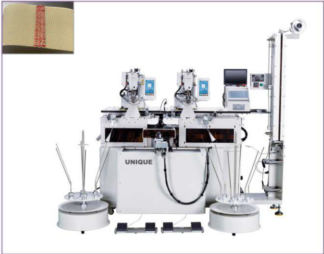
UN-A300B-2-U Full automatic double-station elastic joining machine with auto feeding, ultrasonic cutting and logo positioning. Auto over-knotting and length metering Max. elastic width: 5cm Min. elastic circumstances: 20cm Optional: industrial camera for color sensor
