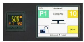
Air pressure digital meter to prevent the malfunctioning of the machine during operation
